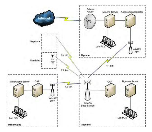
Figure 5.6: SLL - Logical Network Layout - Deployment
