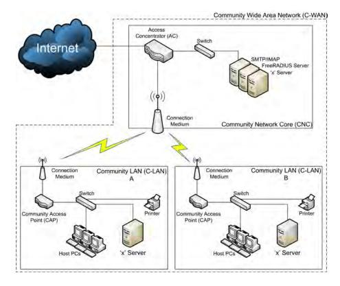
Figure 3.2: Conceptual System Design
