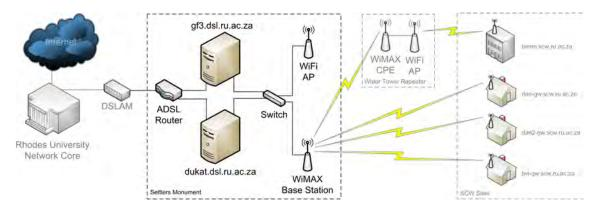
Figure 5.1: CoE Testbed - Logical Network Layout - SCW Deployment
