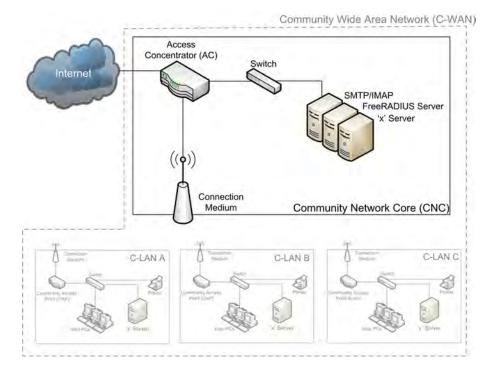
Figure 3.4: Access Concentrator (AC)
