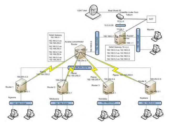
Figure 2.12: SLL - Logical Network Structure
