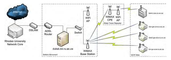
Figure 2.10: CoE Testbed - SCW - Logical Network Structure
