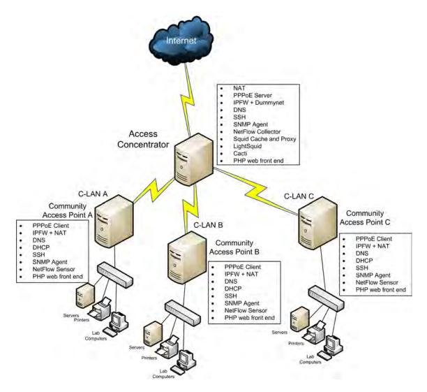
Figure 4.1: Overview of System Developed
