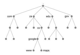
Figure 2.7: Domain Name System (DNS) Tree Structure
